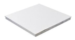
Solid panels specifically designed for Clean Room applications: the unique rib structure provides excellent dispersion of weights to achieve minimum deflection with maximum load- bearing capacities for placement of equipment and tool moves-ins.
