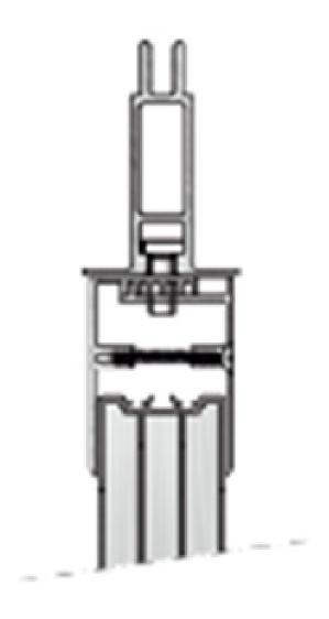
Double clamp-fastened profiles in anodised extruded aluminium, fixed to the filter-holder grid by hammerhead screws.
