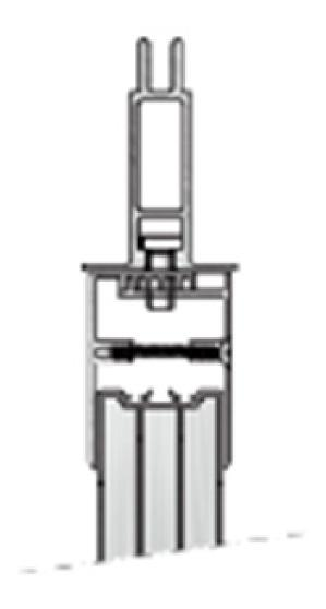
Double clamp-fastened profiles in anodised extruded aluminium, fixed to the filter-holder grid by hammerhead screws.
