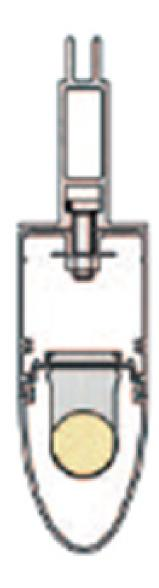
Teardrop light with aerodynamic profile specially designed for use in controlled contamination environments.
