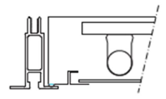
Ceiling light with aerodynamic profile specially designed for use in controlled contamination environments.
