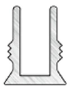
Anodised aluminium profile for closure of the slot of the profile: click-in insertion.
