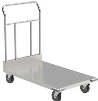
Trolley manufactured in stainless steel AISI 304. Frame in round tube with lower platform in stainless steel sheet 2.00mm thick, reinforced with 3 longitudinal bars. Rear upstand with pull handle, manufactured in stainless steel round tube. On 2 swivels and 2 braked anti-trace castors, diam. 125mm, and with stainless steel frame.
