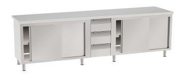
Manufactured in stainless steel AISI 304. Working top in AISI 304 sheet, 1.20mm thick, with inner plywood reinforcement and stainless steel lower cover. Rounded (R=10mm) front upper edge, as well as rounded (R=2mm) side and back edges. Optional rear stainless steel upstand H=100mm,
