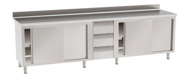
Manufactured in stainless steel AISI 304. Working top in AISI 304 sheet, 1.20mm thick, with inner plywood reinforcement and stainless steel lower cover. Rounded (R=10mm) front upper edge, as well as rounded (R=2mm) side and back edges. Optional rear stainless steel upstand H=100mm,
