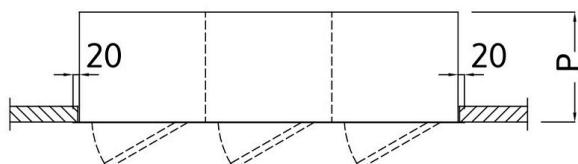
Wardrobe cabinet manufactured in AISI 304 with scotch brite finish. Hinged door mounted on removable hinges, equipped with key lock and upper and lower ventilation holes for air flow. The cabinet is divided into 2 compartments by a vertical partition: clean area and dirty area. Each compartment is equipped with 1 upper shelf with hanging rod and 1 lower shelf, both adjustable in height. On stainless steel telescopic feet, the rear ones advanced for rounded floor.
