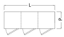
Wardrobe cabinet manufactured in AISI 304 with scotch brite finish. Hinged door mounted on removable hinges, equipped with key lock and upper and lower ventilation holes for air flow. Each compartment is equipped with 1 upper shelf with hanging rod and 1 lower shelf, both adjustable in height. On stainless steel telescopic feet, the rear ones advanced for rounded floor.
