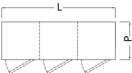
Wardrobe cabinet manufactured in AISI 304 with scotch brite finish. Hinged door mounted on removable hinges, equipped with key lock and upper and lower ventilation holes for air flow. Each compartment is equipped with 1 upper shelf with hanging rod and 1 lower shelf, both adjustable in height. On stainless steel telescopic feet, the rear ones advanced for rounded floor.
