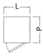
Wardrobe cabinet manufactured in AISI 304 with scotch brite finish. Hinged door mounted on removable hinges, equipped with key lock and upper and lower ventilation holes for air flow. Each compartment is equipped with 1 upper shelf with hanging rod and 1 lower shelf, both adjustable in height. On stainless steel telescopic feet, the rear ones advanced for rounded floor.
