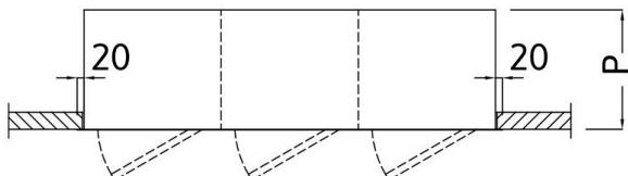
Wardrobe cabinet manufactured in AISI 304 with inner and outer scotch brite finish. Prepared for wall-recessed mounting, with doors profile leveled with the wall. Hinged door mounted on removable hinges, equipped with key lock. Each compartment is equipped with 1 upper shelf with hanging rod and 1 lower shelf, both adjustable in height.
