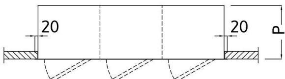
Wardrobe cabinet manufactured in AISI 304 with inner and outer scotch brite finish. Prepared for wall-recessed mounting, with doors profile leveled with the wall. Hinged door mounted on removable hinges, equipped with key lock. Each compartment is equipped with 1 upper shelf with hanging rod and 1 lower shelf, both adjustable in height.
