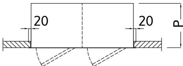
Wardrobe cabinet manufactured in AISI 304 with inner and outer scotch brite finish. Prepared for wall-recessed mounting, with doors profile leveled with the wall. Hinged door mounted on removable hinges, equipped with key lock. Each compartment is equipped with 1 upper shelf with hanging rod and 1 lower shelf, both adjustable in height.
