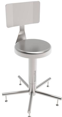
Entirely manufactured in stainless steel AISI 304. Seat Ø 330mm, adjustable in height between 500 and 600mm. Backrest easily adjustable without tools. Supporting base with 5 rays. On stainless steel feet. Completely dismountable for sterilization in autoclave.
