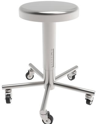
Entirely manufactured in stainless steel AISI 304. Seat Ø 330mm, adjustable in height between 500 and 600mm. Supporting base with 5 rays. Castors Ø60mm on stainless steel frame. Completely dismountable for sterilization in autoclave.
