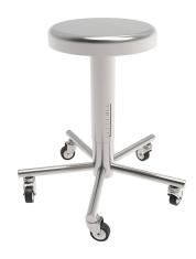
Entirely manufactured in stainless steel AISI 304. Seat Ø 330mm, adjustable in height between 500 and 600mm. Supporting base with 5 rays. Castors Ø60mm on stainless steel frame. Completely dismountable for sterilization in autoclave.
