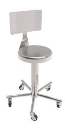
Entirely manufactured in stainless steel AISI 304. Seat Ø330mm, adjustable in height between 500 and 600mm. Backrest easily adjustable without tools. Supporting base with 5 rays. Castors Ø60mm on stainless steel frame. Completely dismountable for sterilization in autoclave.
