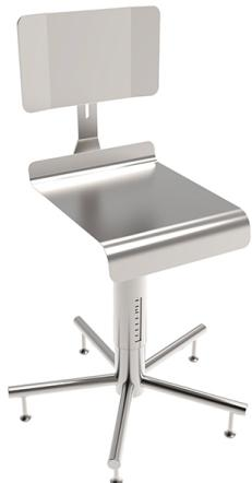
Entirely manufactured in stainless steel AISI 304. Seat dim. 380x400mm, adjustable in height between 500 and 600mm. Backrest easily adjustable without tools. Supporting base with 5 rays. On stainless steel feet. Completely dismountable for sterilization in autoclave.
