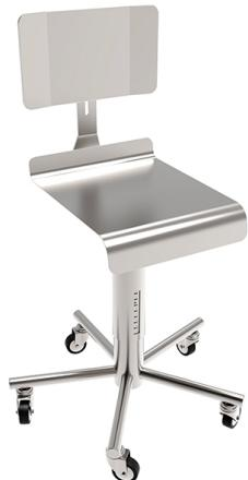
Entirely manufactured in stainless steel AISI 304. Seat dim. 380x400mm, adjustable in height between 500 and 600mm. Backrest easily adjustable without tools. Supporting base with 5 rays. Castors Ø60mm on stainless steel frame. Completely dismountable for sterilization in autoclave.
