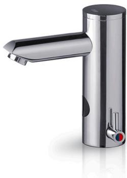
Electronic faucet equipped with photocell sensors. Water temperature control via built-in mixing lever. 3x1.5V batteries in watertight box and LED signaling low batteries. Overflow device. Water connections type 1/2 G.
