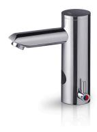
Electronic faucet equipped with photocell sensors. Water temperature control via built-in mixing lever. 3x1.5V batteries in watertight box and LED signaling low batteries. Overflow device. Water connections type 1/2 G.
