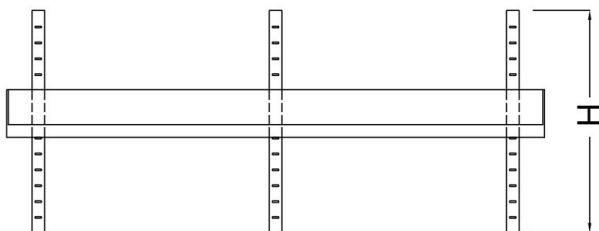
Three shelf rack manufactured in stainless steel AISI 304. Prepared for wall mounting and used as an alternative to the horizontal bar that comes with the shelf, allowing height adjustment.
