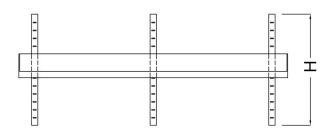
Three shelf rack manufactured in stainless steel AISI 304. Prepared for wall mounting and used as an alternative to the horizontal bar that comes with the shelf, allowing height adjustment.
