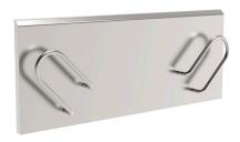
Manufactured in stainless steel AISI 304. With 2 rounded hooks in AISI 304 bended Ø8mm round wire, meant for hanging tubes to drip. Wall mounting stainless steel screws included. Length 500.
